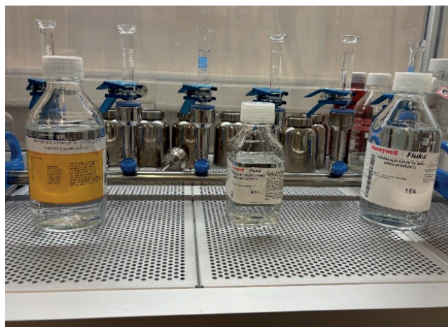
Figure 1: Sample filtration setup in a laminar flow cleanbench.
